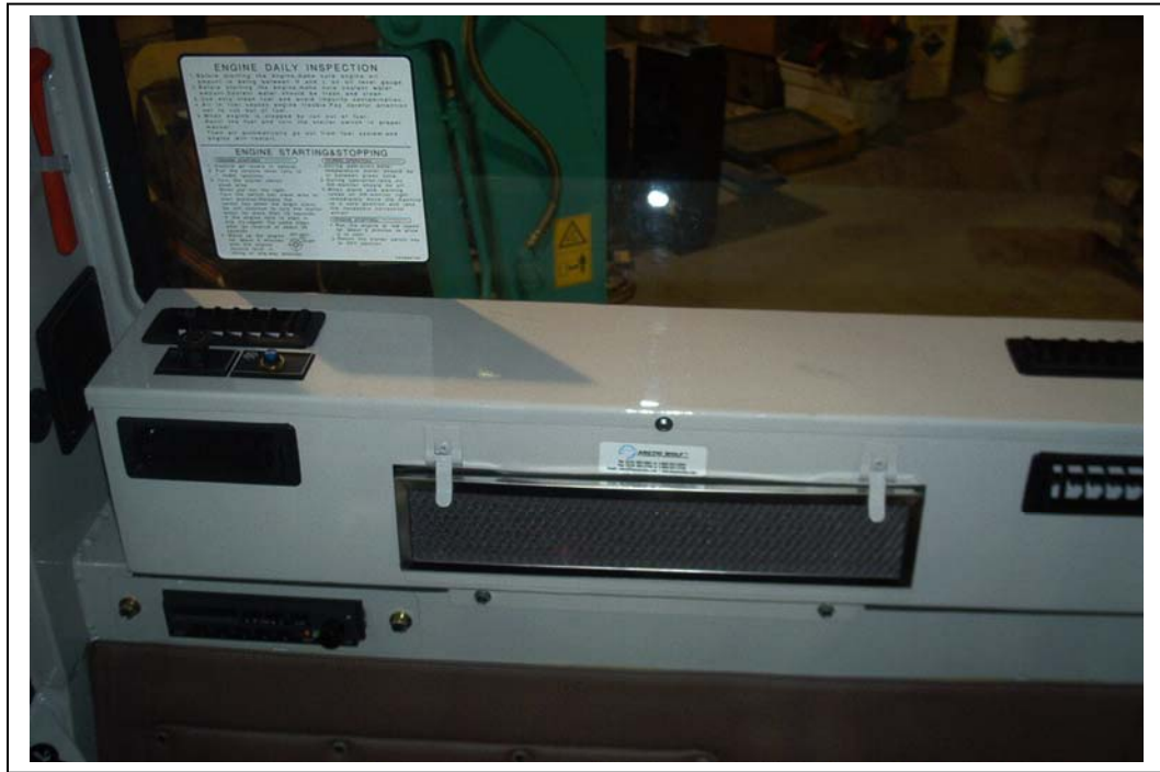
Evaporator mounted in cab behind operator seat.
